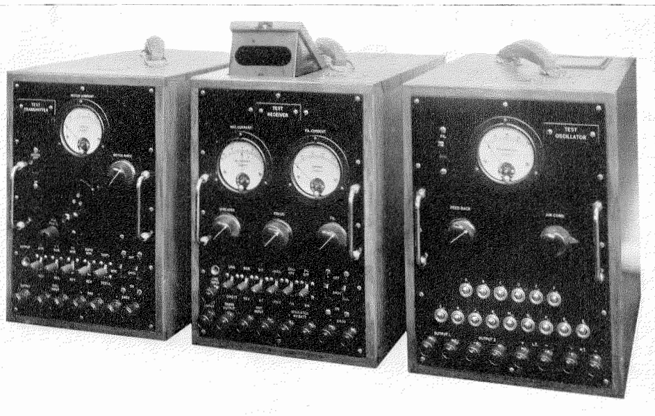
Figure 8—Complete Telegraph Distortion Measuring Set.
